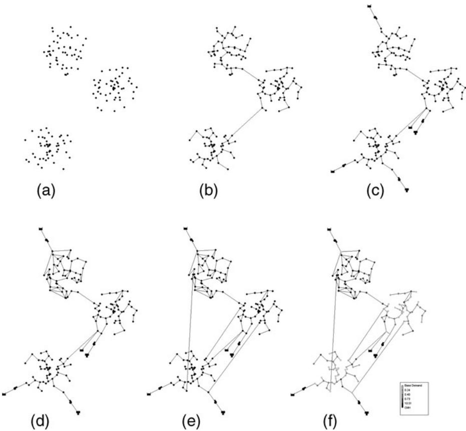
**Fig. 2** Stepwise generation of (a) clusters; (b) tree structure, (c) reservoirs, tanks, pumps; (d) intra-cluster pipes; (e) inter-cluster pipes; (f) base load and demand patterns
