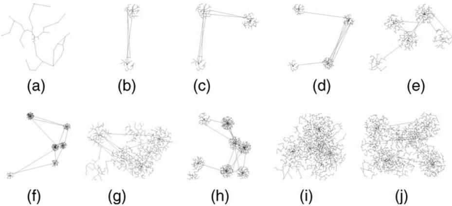
**Fig. 6** HydroGen examples with varying distance parameters: **(a)** 1 cluster of 50 nodes; **(b)** 2 clusters of 50 and 100 nodes; **(c)** 3 clusters of 50, 100 and 150 nodes; **(d)** 4 clusters of 50 to 200 nodes; **(e)** 5 clusters of 50 to 250 nodes; **(f)** 6 clusters of 50 to 300 nodes; **(g)** 7 clusters of 50 to 350 nodes; **(h)** 8 clusters of 50 to 400 nodes; **(i)** 9 clusters of 50 to 450 nodes; **(j)** 10 clusters of 50 to 500 nodes
