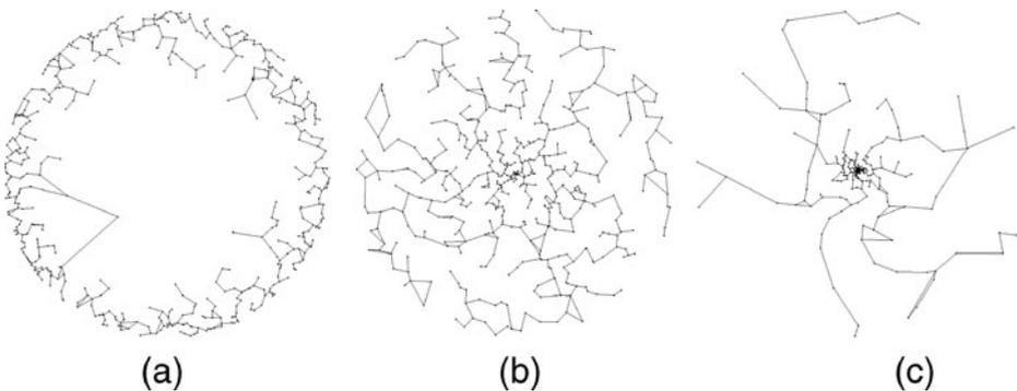
**Fig. 3** HydroGen examples of a network of 500 nodes with cluster type 3 and varying  $d$ -factor: (a)  $d = 0.1$ ; (b)  $d = 1$ ; (c)  $d = 10$
